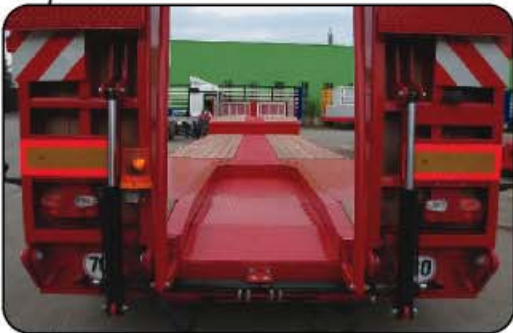
Excavator through for easy transport of vehicles with long booms
