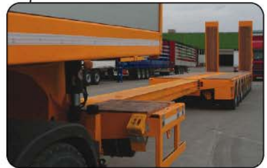
Extending loading platform
